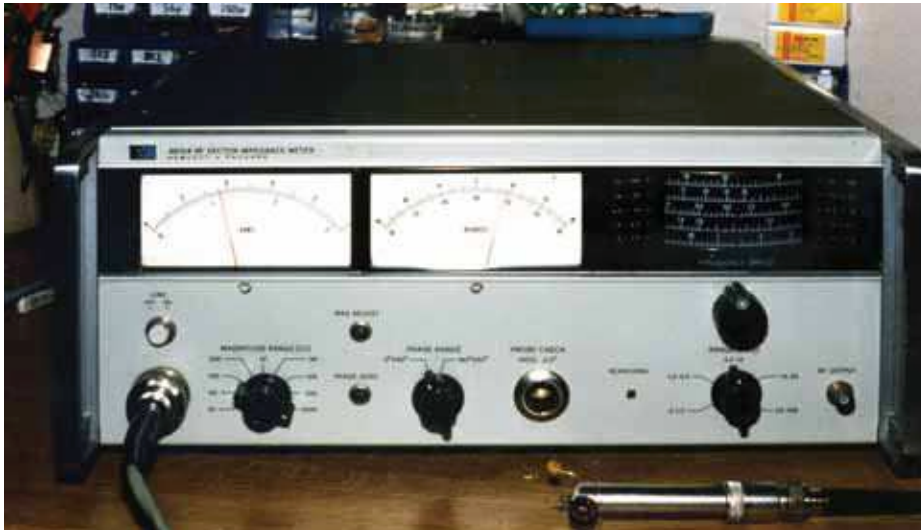
PHOTO 1: HP4085 vector impedance meter. The meter on the left indicates Z_{mag} in ohms while the right hand meter indicates Theta in degrees.
